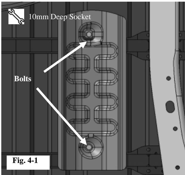
**4. Remove and Install Heat Shield.**
